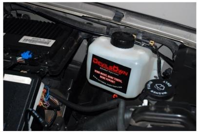
Figure 1: Tank Placement
